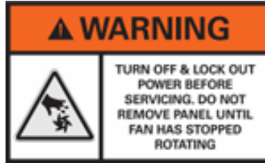
Danger of cuts! Completely disconnect the chiller power supply before opening this cover
